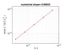
Figure 2: Experimental rate of convergence for cnoidal-wave solution
