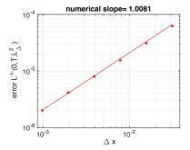
Figure 1: Experimental rate of convergence for sinusoidal solution
