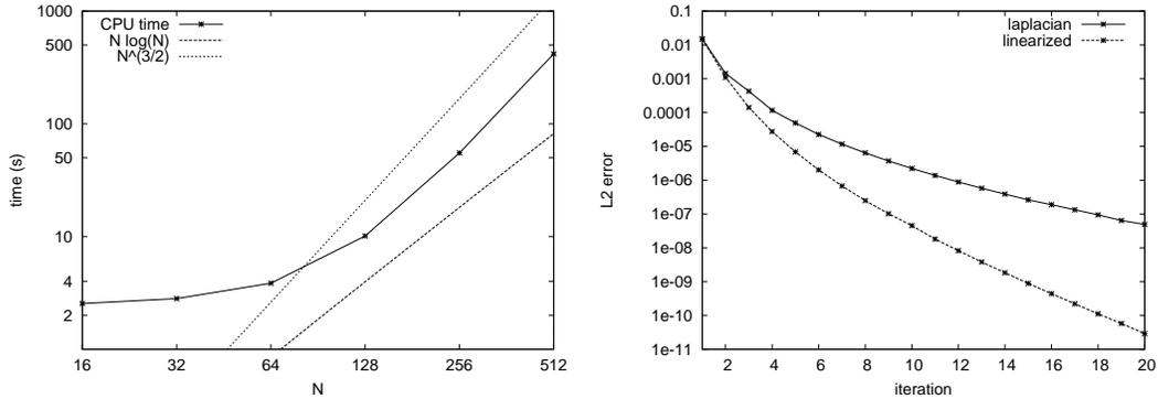
Figure 3. (Left) CPU time in logarithmic scale for the *algorithm* with respect to  $N$  ( $\beta = 0.8$ ,  $k = 2$  and  $\tau = 1$ ). (Right) Convergence history of the error on  $\rho$  ( $\beta = 0.99$  and  $k = 1$ ) in the  $L^2$ -norm over 20 iterations. The Laplace and the linearized Monge-Ampère equations are solved with  $N = 128$  and  $\tau = 1$ .
