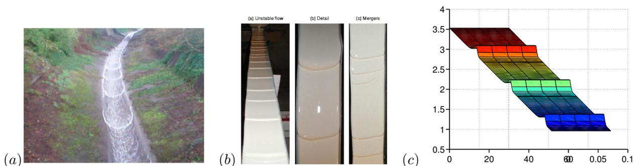
FIGURE 1. Roll waves (a) on a spillway and (b) in the lab: pictures courtesy of Neil Balmforth, UBC. (c) Periodic profile of (1.1),  $F = \sqrt{6}$ ,  $\nu = 0.1$ ,  $q = 1.5745$ ,  $X = 17.15$ . For better comparison to experiment, we extended the profile here as constant in transverse direction.
