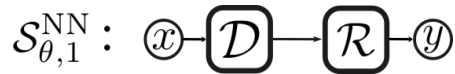
FIGURE 2. Definition of \mathcal{S}_{\theta,1}^{\text{NN}} where \mathcal{D} represents a convolution neuron (or diffusion neuron in reference to diffusion operators), and \mathcal{R} represents a multilayer perceptron (called reaction network in reference to reaction operators). The parameter \theta is the vector of learning parameters, it contains all weights of the \mathcal{D} and \mathcal{R} networks.
