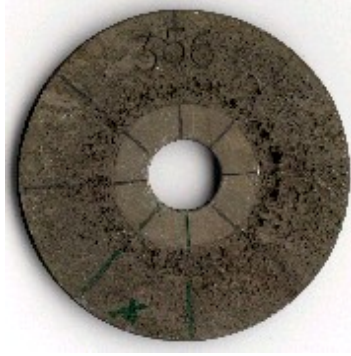
Figure 4: A magnesium plate with pitting corrosion, divided into eight sub-sections for measuring the maximum pit depth in each of the section.
