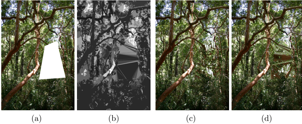
FIG. 8.4. A case where the geometrical guiding yields worst results than the "patchwork" algorithm [71]. In this case, the macro-texture structure is too complex to be correctly interpolated. (a) occluded 676 \times 1014 image (occlusion size \sim 100 \times 300 ); (b) Interpolated sketch using straight lines; (c) image restored using the exemplar-based method from [71]; (d) image restored using the method introduced in this paper, detailed in Section 6 (using p = 4 , q = 6 , \lambda = 0.5 ).
