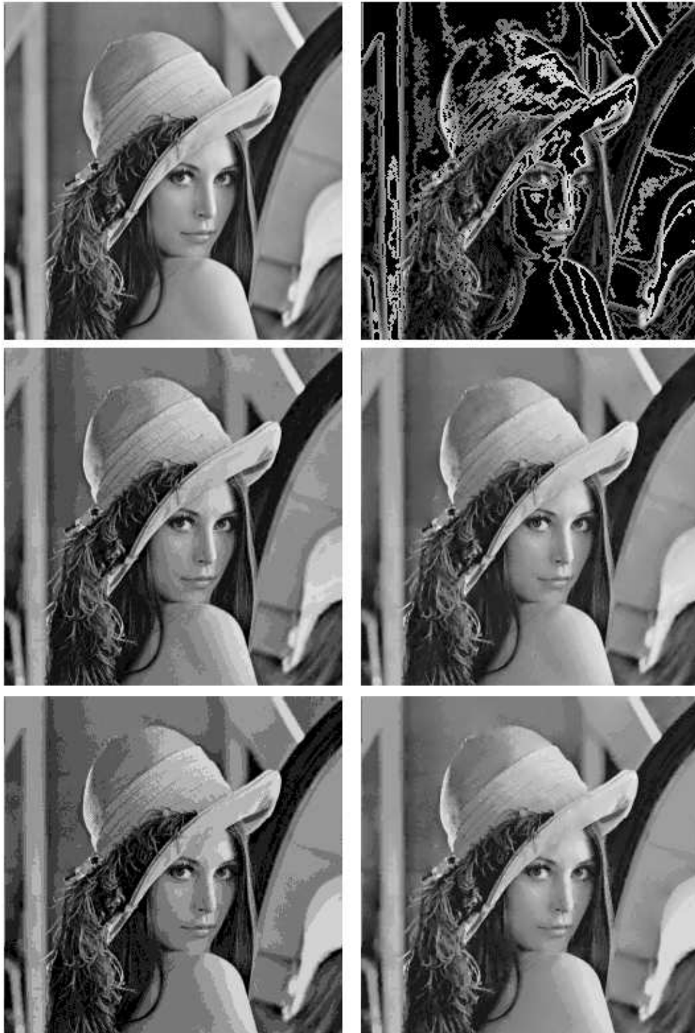
Figure 7: Left top (a): original image – Right top (b): level lines for \delta = 30 . Left middle (c): quantized image for \delta = 20 – Right middle (d): the interpolant for \delta = 20 . Left bottom (e): quantized image for \delta = 30 – Right bottom (f): the interpolant for \delta = 30 .
